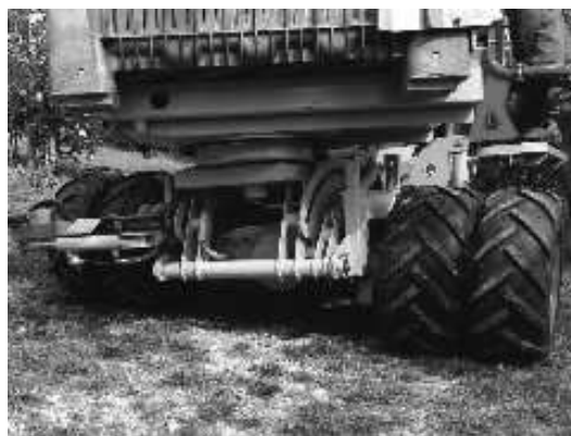
Fot. 3. Elektrohydrauliczny system jezdny „Pluk-O-Traka” [ www.x-lab.it/meccanicazucal/img/as_collina01.jpg ] Pic. 3. Electro-hydraulic suspension system of „Pluk-O-Trak” [ www.x-lab.it/meccanicazucal/img/as_collina01.jpg ]
