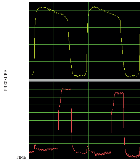
Fig. 8. Indicatory diagram with extended cycle of sucking in one pair of teat cups
