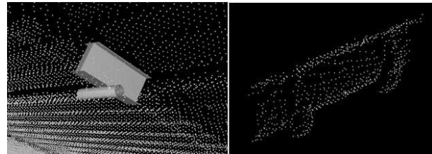
Fig. 5. Modelled node – connection of rope and I-section (left side), detailed part of node in cloud of points with resolution of 2 mm (right side)
